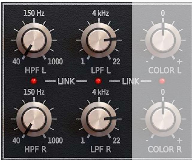
Filter cut-off frequencies for both stereo channels
