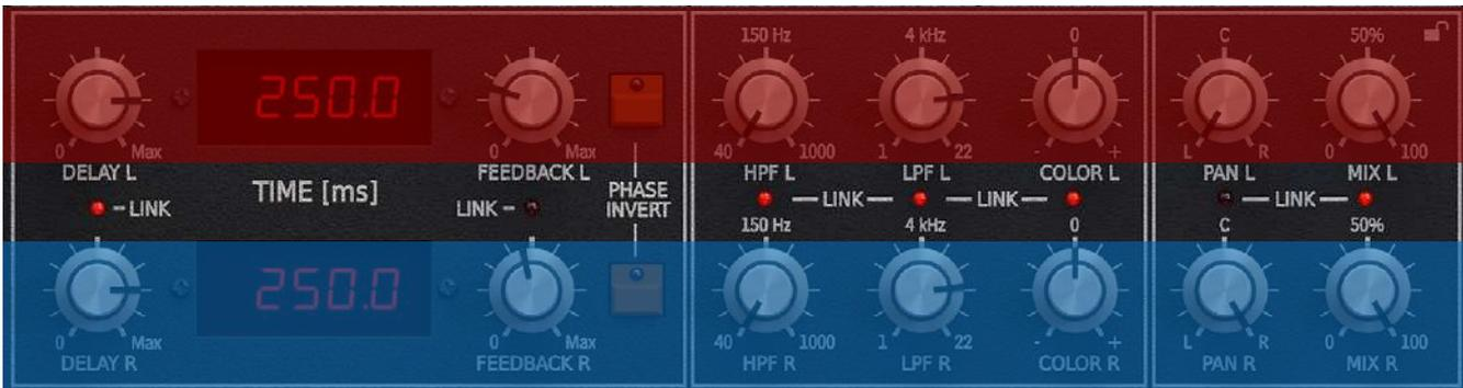
The upper row controls the left channel parameters and the bottom row – the right channel.
