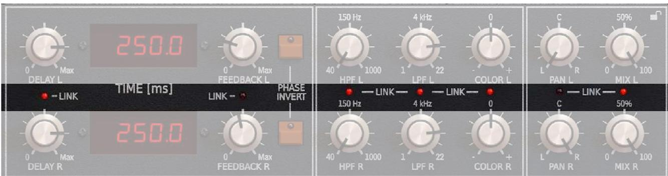
Link LEDs row to join the controls in pairs (left - right channel)
